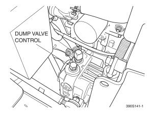
Figure 4-4. Dump Valve Control
